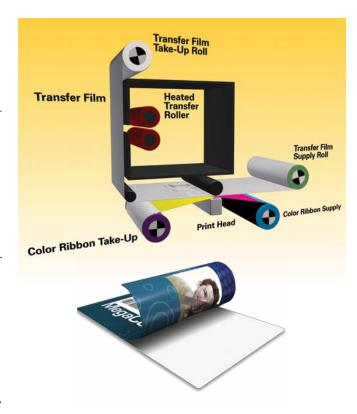
Zebra's patent-pending simultaneous dual-sided image transfer process applies film to both sides of the card in a single pass, drastically reducing the print time.
